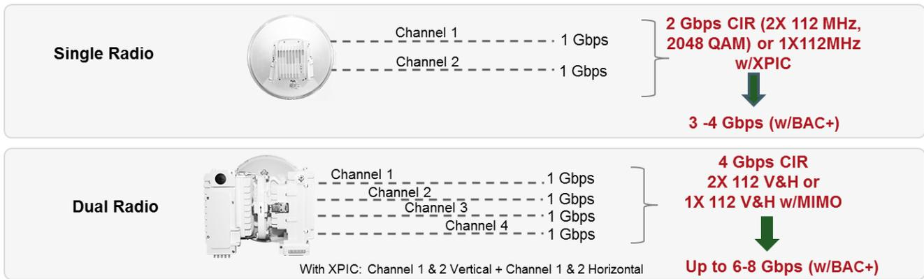
**Figure 1: Single vs. Dual Carrier Configuration**
