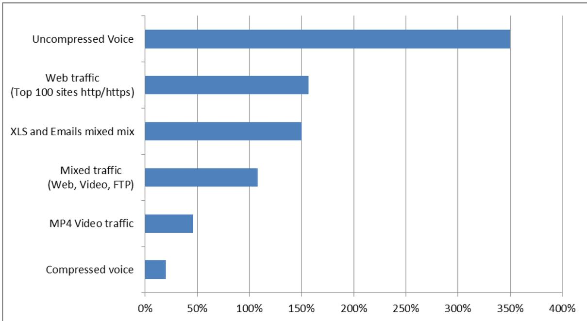
Figure 2: DragonWave Bandwidth Accelerator Performances for Traffic Types
